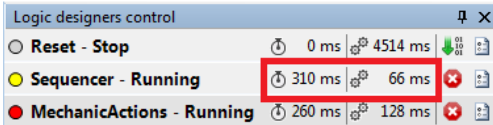
Figure 60: Display of the Last Cycle Interval
